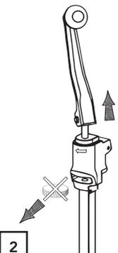
**2** Lift the handle out and wipe shaft clean. Remove the wheel from the chamber.
