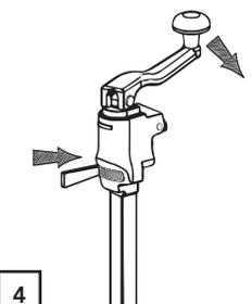
**4** Insert handle and push down firmly to reconnect. Place metal rod in the back left hand side and wind the handle clockwise until you feel it lock but don't over tighten.
