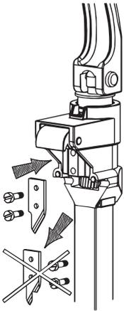
Loosen screws to free blade. Replace the blade and ensure stamped side faces trigger mechanism. Replace screws and tighten.
