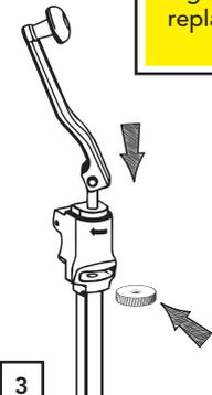
**3** Replace with a new wheel ensuring the Bonzer® text side is facing downward (label on wheel must face upwards)
