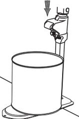
**3** Use palm of hand to push the can opener down firmly, ensure the blade has pierced the can.
