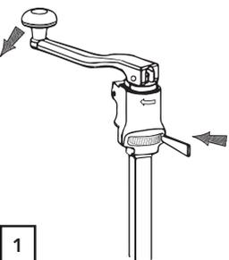
**1** Engage the handle into operational mode (down position). Place the metal rod (provided with new wheel) in the back right hand side of the wheel and wind the handle anticlockwise until loose.
