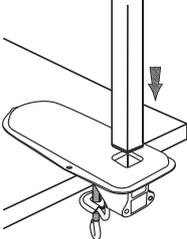
**2** Push can opener shaft down into the base hole.
