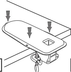
**1** Firmly affix the can opener base to a flat surface with screws and (or) clamp provided.
