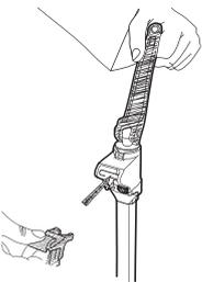
**4** Replace the trigger while pulling back handle.
