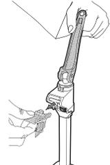
**2** Remove the trigger while pulling back handle.
