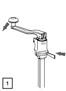
Engage the handle into operational mode (down position). Place the metal rod (provided with new wheel) in the back right hand side of the wheel and wind the handle anticlockwise until loose.
